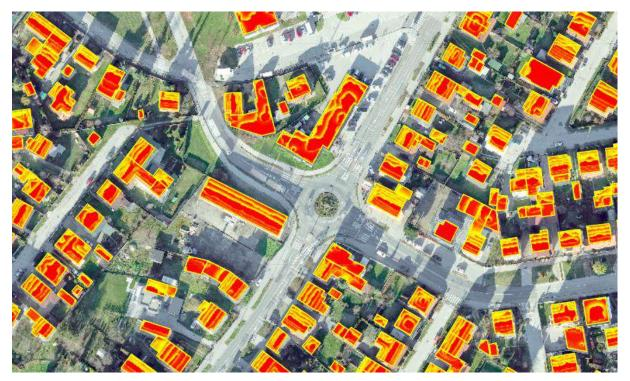
Figure 5 Solar potential map example<sup>7</sup>
