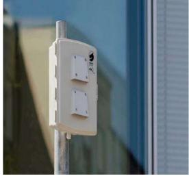
Figure 3 Air Quality Monitoring Device
